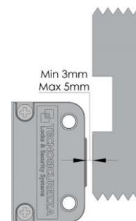
The latch version (Motor LatchBolt lock) is specially designed to ensure self-locking when the door closes.
