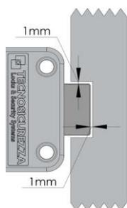
In the locked position, there should be approximately 1 mm clearance between the lock bolt and the cavity in the blocking bar of the boltwork. The bolt must be able to move freely without force being applied to it.
