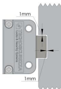
In the locked position, there should be approximately 1 mm clearance between the lock bolt and the cavity in the blocking bar of the boltwork. The bolt must be able to move freely without applying any force on it.
