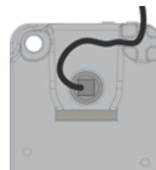
Connect the keypad cable to the lock connector "1", making sure it is fully inserted and locked. Any alarm interface or battery holder needs to be connected to the lock connector "2". To remove the cable, bring the connector upwards and carefully pull it out.
