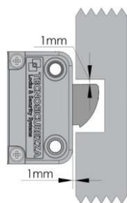
In the locked position the distance between the lock's bolt and the lock part that moves the lock bolt should be approximately 1 mm.
