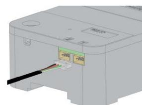
The Push & Pull version (T5101/MP) is supplied by default with RCS option, where closing is triggered by an external signal (i.e. boltwork switch). This avoids the motor to be activated when boltworks are not expanded yet.
