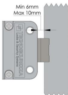
The distance between the lock and the locking edge must be between a minimum of 6 mm and a maximum of 10 mm.
