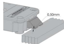
Cut the spindle to the correct length (measure door thickness + mounting plate/rotation knob or handle insert + lock spindle insert).
