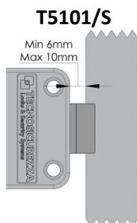
The distance between the LatchBolt lock and the locking edge must be between a minimum of 6 mm and a maximum of 10 mm.
