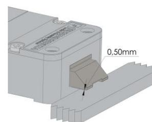
Insert the keypad cable into the lock connector "1", making sure it is fully inserted and locked.
