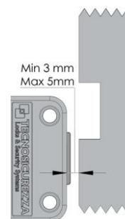
The maximum load applicable to the bolt must not exceed 1 KN. Contact Tecnosicurezza in case of heavier loads.
