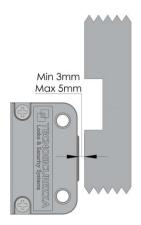
The Motor LatchBolt lock is specially designed to ensure self locking when the door closes.
