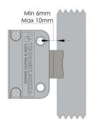
The distance between the lock and the locking edge must be between a minimum of 6 mm and a maximum of 10 mm.
