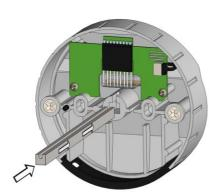
Fix the screws (M4) and the rotating backplate, positioning the latter on the side marked "UP". Fix the bushings to the keypad housing using the supplied screws.
