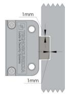
In the locked position, there should be approximately 1 mm clearance between the lock bolt and the cavity in the blocking bar of the boltwork. The bolt must be able to move freely without applying any force on it.
