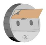
Remove the release liner placed under the membrane and apply the latter on the keypad case.
