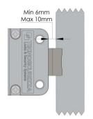
The distance between the LatchBolt lock and the locking edge must be between a minimum of 6 mm and a maximum of 10 mm.
